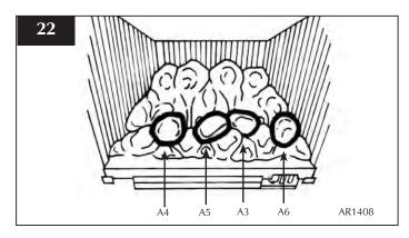
8.15 Place the next four pebbles as identified resting between the flame baffle and the first row of pebbles as shown in Diagram 23.
